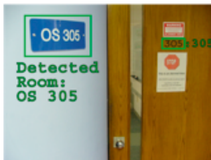
In this simulated example, optical character recognition detects the room number. Reading room numbers is a complex task because any number is just as likely to be followed by any of the ten digits and possibly a dash, punctuation or letters.
