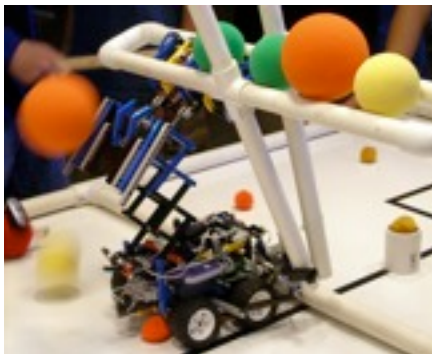
A robot with its "puncher" extended. This design was one of many ways to solve the open-ended 2006 Botball challenge.
