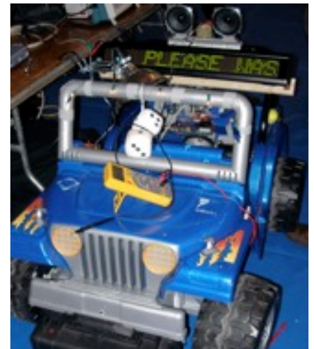
MCP, a PowerWheels jeep turned robot, began as a Robotics I final project in Spring 2004. MCP is now the focus of the graduate Robot Design class.
