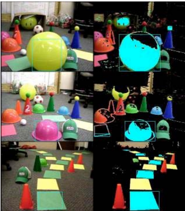
Figure 6: (a) Histogramming yellow ball and (b) HSV Threshold and blobbing yellow ball. (c) Histogramming the pink Bowl and (d) HSV Threshold and Blobbing of the pink bowl. (e) Histogramming a sheet of green paper on the floor and (f) HSV Threshold and blobbing of the green paper laid in a trail.
