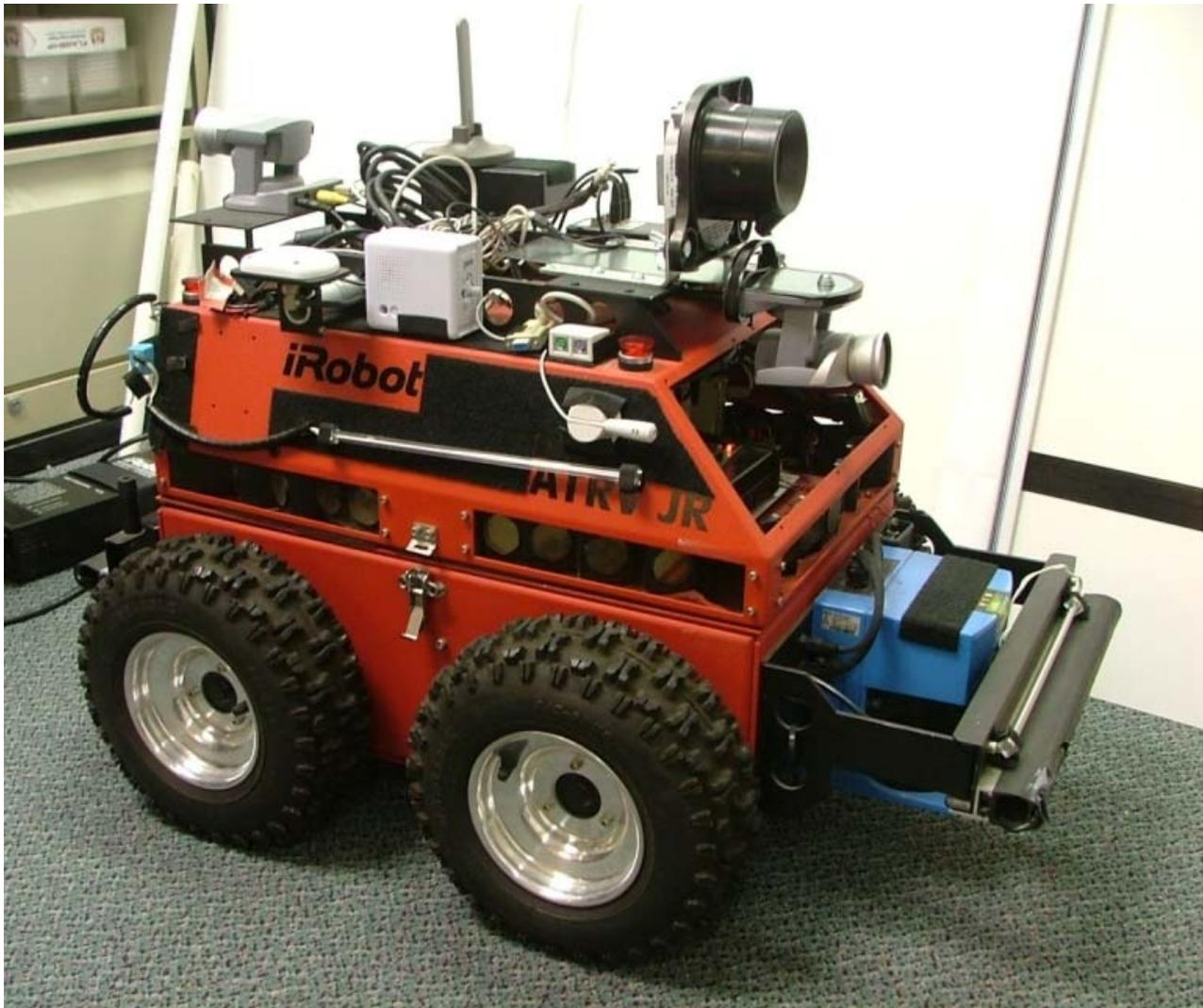
**Figure 3-1.** iRobot ATRV-Jr robot.
