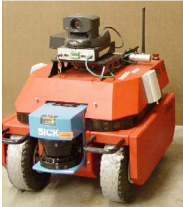
Figure 1: The INL robot: an iRobot ATRV-Mini
