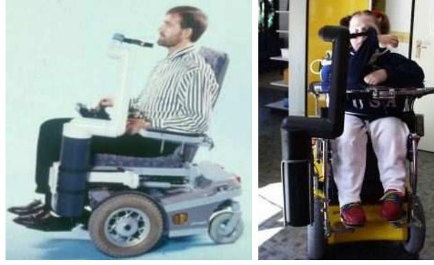
Figure 26. The Manus ARM was typically mounted over the front wheels of a power wheelchair. Left and right Manus ARMs are shown left and right, respectively. (from Exact Dynamics 2008)
