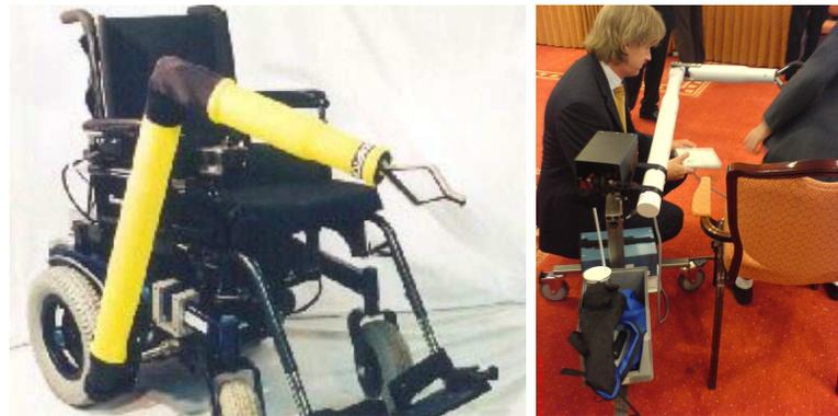
Figure 13. The Raptor Wheelchair Mounted Robotic Arm (from Phybotics 2008). The Raptor exhibited at ICORR'07 (Courtesy of Michelle Johnson).
