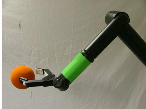
Figure 31. The indirect selection interface system used color tracking to move the Manus ARM.
