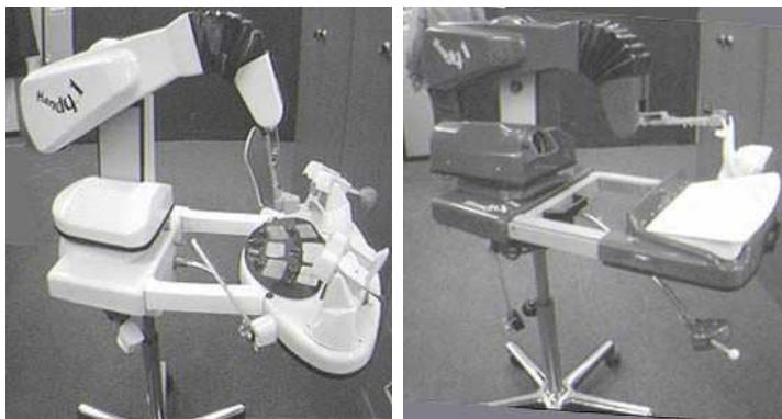
Figure 3. Kale University's Handy 1 feeding aid features a Cyber 310 robot arm (from Fazakerley 2006).
