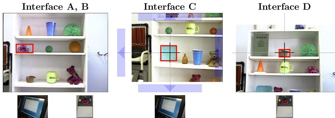
Figure 37. Object selection using our direct selection interface. The fixed camera view selection is shown on the left. The moving camera view is shown center and right, using touch screen and joystick, respectively.
