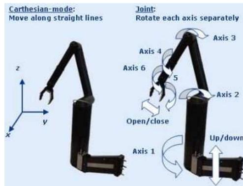
Figure 27. The Manus ARM was controlled by moving its joints independently or by moving the gripper linearly through Cartesian space. (from Exact Dynamics 2008)
