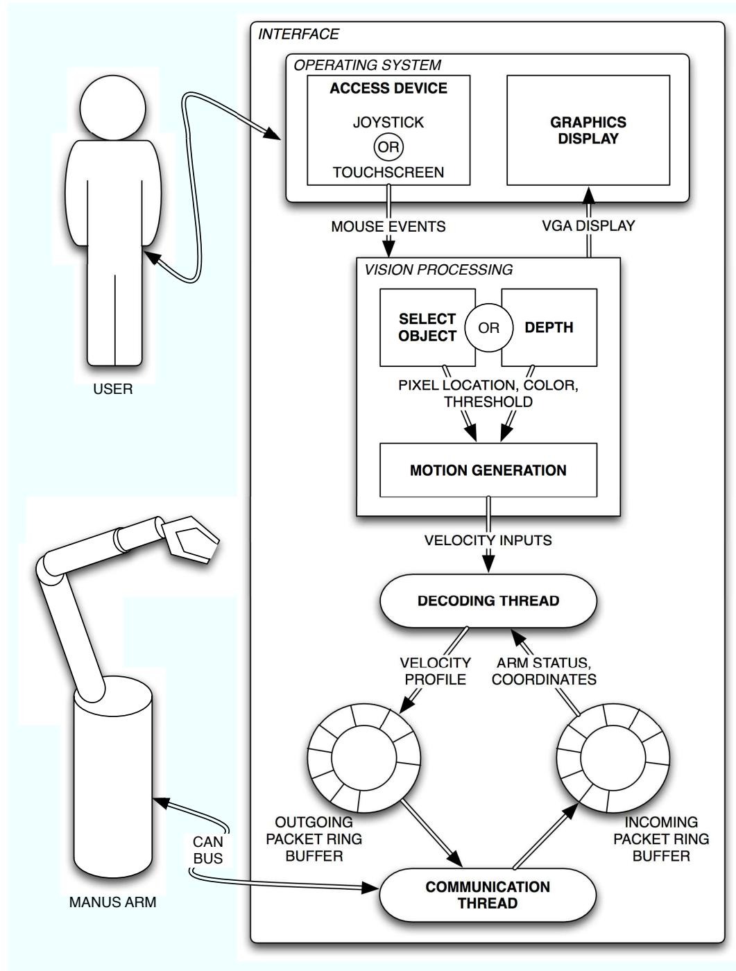
Figure 30. Data flow of our direct selection human-in-the-loop visual control system for the Manus ARM. The user provided input via touch screen or joystick mouse (top). The input was used in the vision processing (center) to position the robot arm (bottom).
