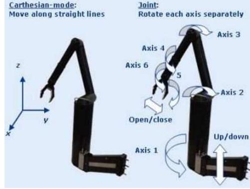
Figure 27. The Manus ARM was controlled by moving its joints independently or by moving the gripper linearly through Cartesian space. (from Exact Dynamics 2008)
