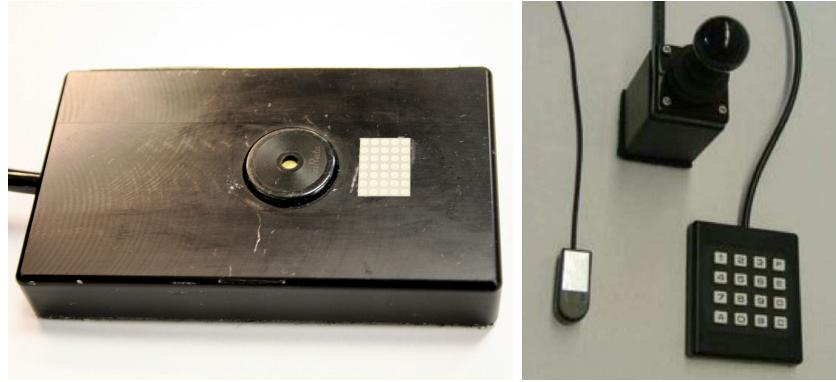
Figure 22. (Left) Feedback of the robot arm’s current status was shown in a  $5 \times 7$  LED matrix and piezo buzzer. (Right) The Manus ARM was controlled manually with a keypad, joystick, or single switch.
