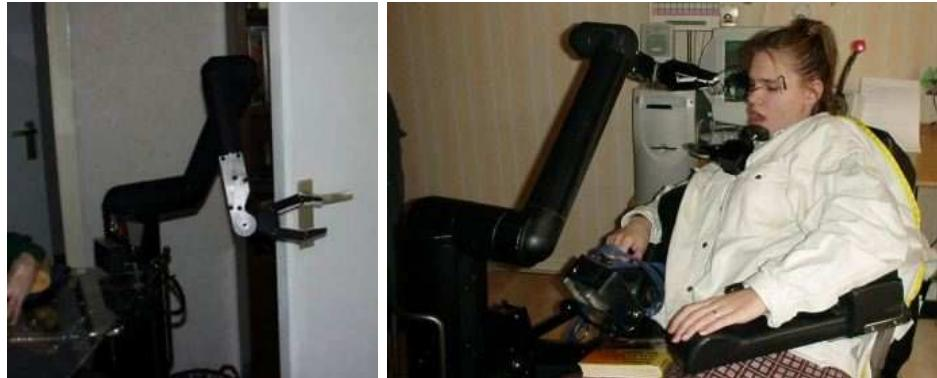
Figure 14. The Manus Assistive Robotic Manipulator can assist in activities of daily living, such as operating door handles and putting on glasses (from Exact Dynamics 2008).
