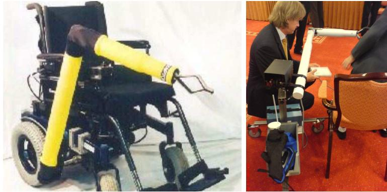
Figure 13. The Raptor Wheelchair Mounted Robotic Arm (from Phybatics 2008). The Raptor exhibited at ICORR'07 (Courtesy of Michelle Johnson).
