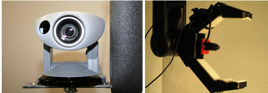
Figure 28. (Left) A Canon VC-C50i on the “shoulder” of the Manus ARM approximated the wheelchair occupant’s view. (Right) A camera mounted within the gripper provided an up close view of the object to be grasped.
