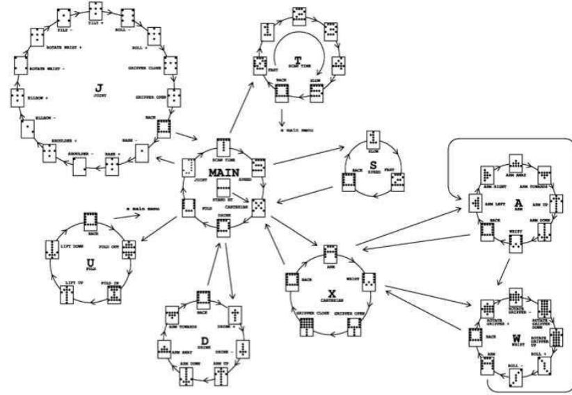
Figure 25. The Manus ARM's single switch menu was two or three layers deep depending upon the desired functionality and may interconnect between submenus. The timing component inherent to single switch applications was indicated as a clockwise cycle. (Courtesy of Exact Dynamics)
