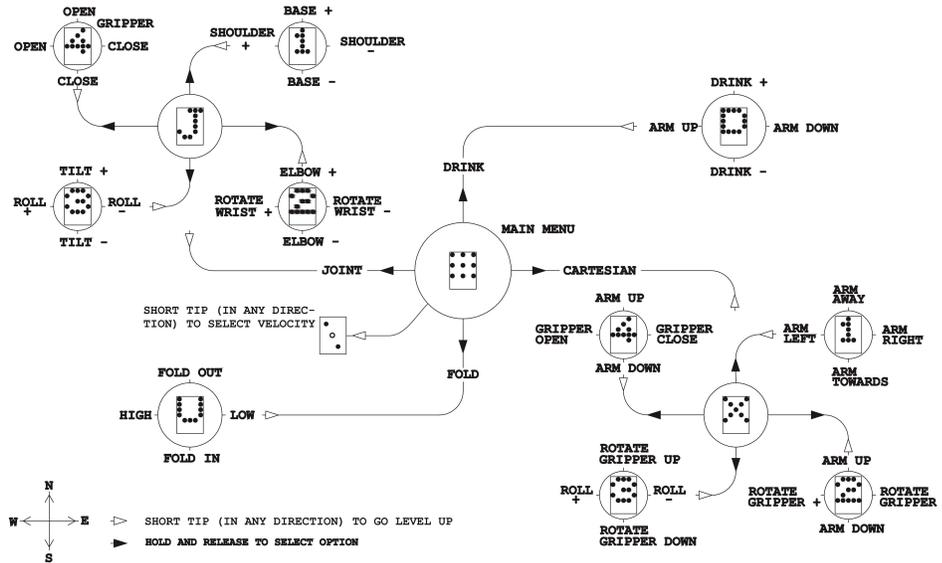
Figure 24. The Manus ARM’s joystick menu was three layers deep to move in joint or Cartesian mode. To access a submenu, the user quickly tapped the joystick in the corresponding direction. (Courtesy of Exact Dynamics)
