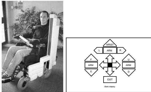
Figure 7. The Bath Institute of Medical Engineering's Weston robot arm is shown on the left, and graphical user interface shown on the right. (from Hillman et al. 2002)
