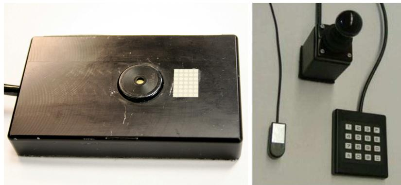
Figure 22. (Left) Feedback of the robot arm's current status was shown in a  $5 \times 7$  LED matrix and piezo buzzer. (Right) The Manus ARM was controlled manually with a keypad, joystick, or single switch.
