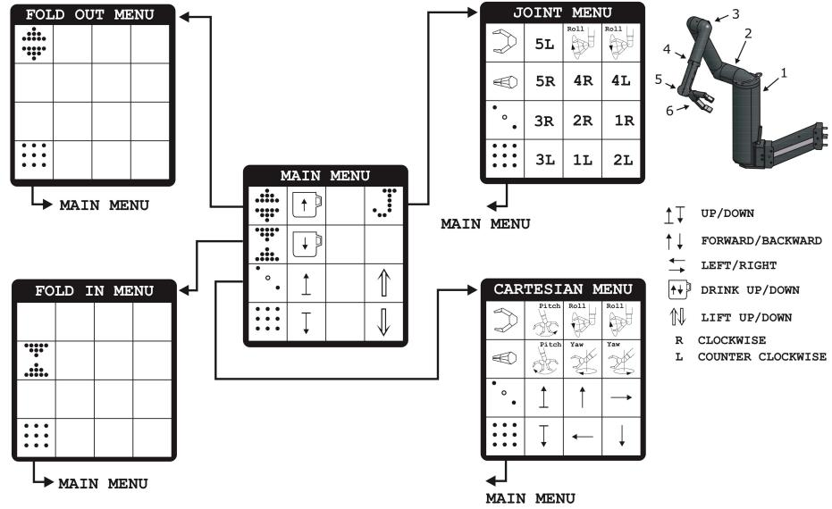
Figure 23. The Manus ARM's keypad menu was two layers deep for all functionality. The menus corresponded directly to the  $4 \times 4$  alpha-numeric keypad. (Courtesy of Exact Dynamics)
