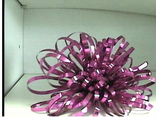
Figure 33. A view from the gripper camera after “dropping in” for depth  $Z$ . The gripper was well within twelve inches from the object.
