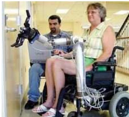
Figure 5. University of South Florida's 7 degree of freedom robot arm (from Higgins 2007)
