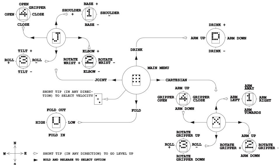
Figure 24. The Manus ARM's joystick menu was three layers deep to move in joint or Cartesian mode. To access a submenu, the user quickly tapped the joystick in the corresponding direction. (Courtesy of Exact Dynamics)
