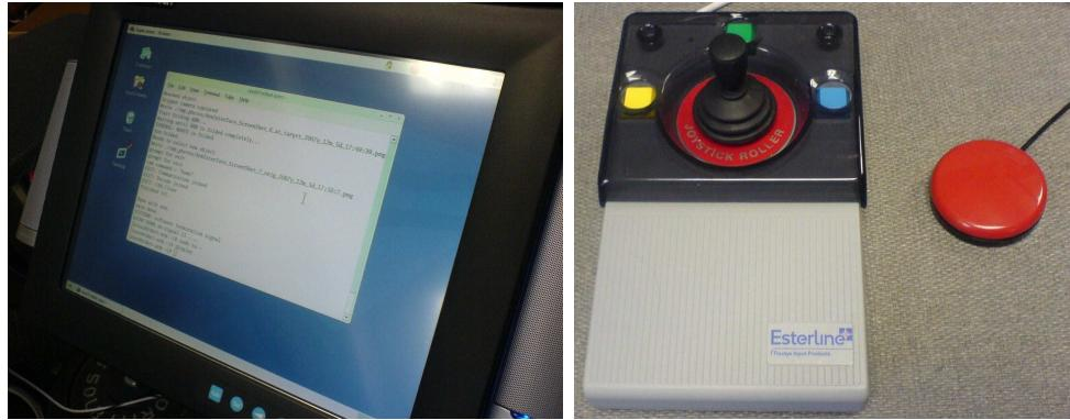
Figure 29. Our visual interface utilizes commonly used assistive technology devices such as a touch screen (left), joystick (right), and jellybean switch (far right).
