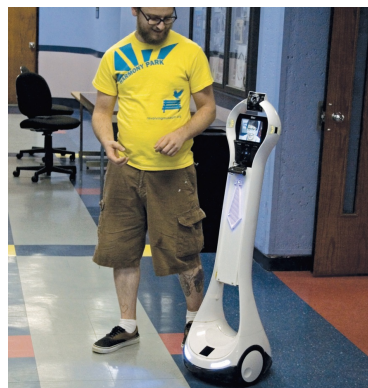
Figure 1: Hugo (an augmented VGo Communication's VGo telepresence robot) is being driven remotely and being used to walk alongside a colleague, actively participating in a mobile conversation. The driver can be seen on Hugo's screen.
