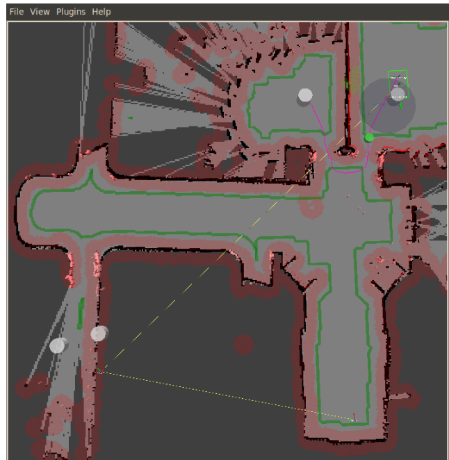
Figure 4: The robot generates a map of the environment in a frontier-based exploration scenario.
