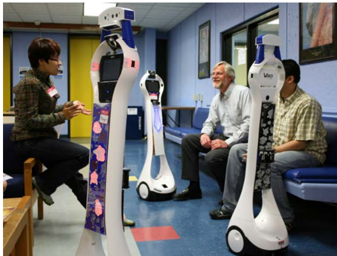
Fig. 1. Margo (left robot) showing the front view of our v1 design with Hawaiian shirt and tricolor LEDs. Back panel is shown on a sibling v1 robot, Largo (right). Hugo (center), v0 prototype, features a blue LED necktie.
