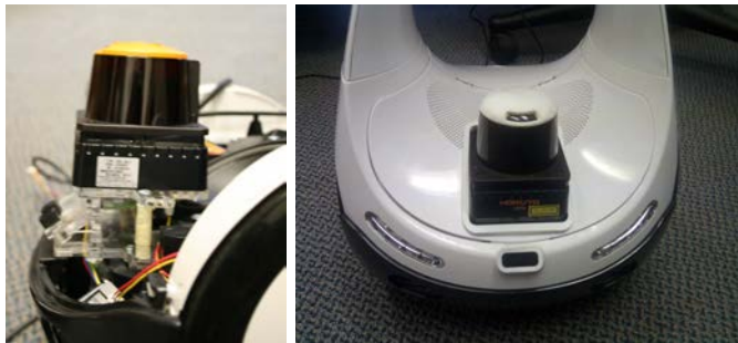
Fig. 4. (Left) The Hokuyo UGH-08 laser is mounted in the forward center of the VGo robot's base over the base speaker. (Right) The laser's formerly orange cap has been covered with white silicon Sugru to visually minimize it.
