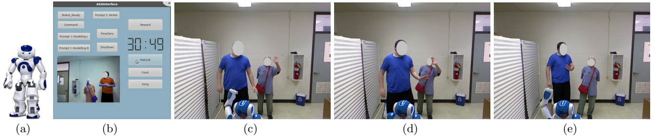
Figure 2: (a) The humanoid robot ‘Blue’ (Aldebaran Robotics Inc.) (b) The robot-control interface (c-e) The modeling prompt is helping the participant P1 (on the left) to gradually execute the correct behavior
