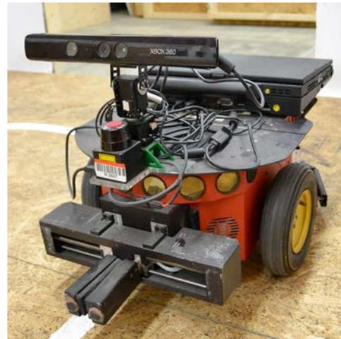
**Figure 6.** The Adept MobileRobots Pioneer 3 with additional sensors.
