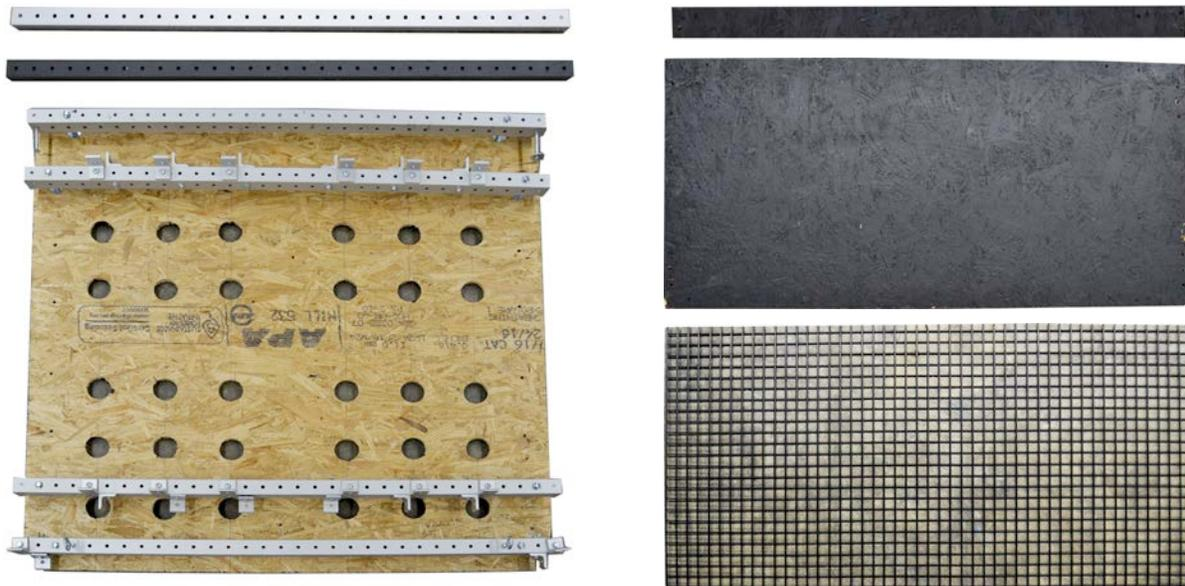
**Figure 3.** The common building materials used to fabricate the obstacle test props. Left, top to bottom: aluminum square tubing, black square tubing, horizontal plane with holes and hardware for mounting additional components. Right, top to bottom: thin solid panels, tall solid panels, mesh side panels.
