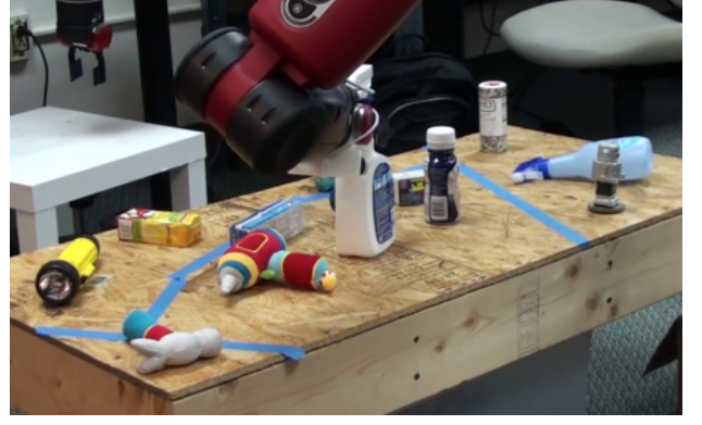
Fig. 5. Experimental scenario for evaluating the grasping system by itself.
