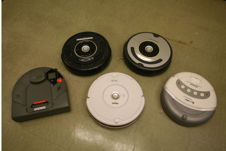
Figure 14.4: The set of robots used in the experiment, with four Roomba models and one Neato robot. Neato (far left) and the Discovery model Roomba (far right) were disabled to include “broken” robots in the experiment design.
