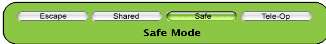
Figure 10: The mode panel shows the current autonomy mode the robot is in. The background color and highlighted button will change depending what mode the robot is in.
