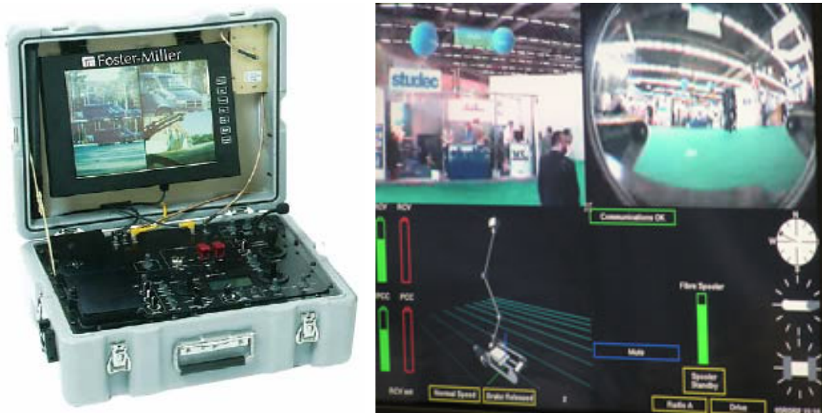
Figure 5: On the left is the Foster-Miller Talon robot's operator control unit. It consists of four video displays from various cameras on the robot. On the right is the iRobot Packbot EOD interface. It contains video streams from the main camera on the top left and a video window on the top right that can display video streams from other cameras located on the system. It also shows the current mechanical arm position, as well other status information. Photos from: http://www.electronicdesign.com/Files/29/14132/Figure_02.jpg . and http://www.defense-update.com/products/p/pacbot.htm
