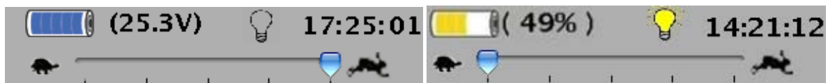
Figure 11: The status panel. Generally the information is not mission critical, but it is good to have access. This information includes battery life, the lighting system status, current time and the max speed setting of the robot.
