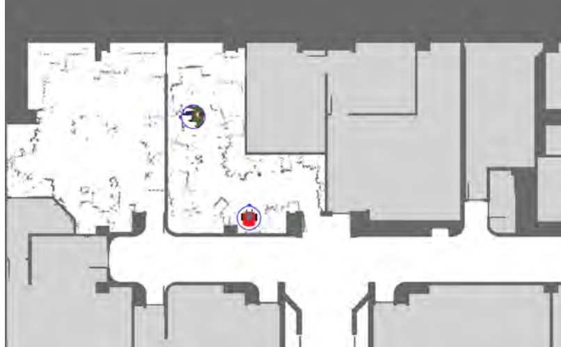
Figure 4-2: Screenshot of command system displaying a person alongside a robot on a section of a pre-generated map. The map was built from the combination of a floor plan and robot laser sensor input. Varying shades of gray on the map represent probabilities of an obstacle being in a determined location.
