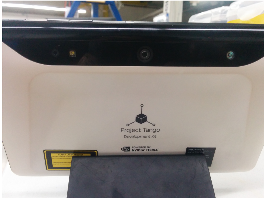
Figure 3-3: Project Tango tablet sensor detail Left to right in the top black bar: Infrared Camera, LED Flash, Fisheye Camera, Infrared Emitter
