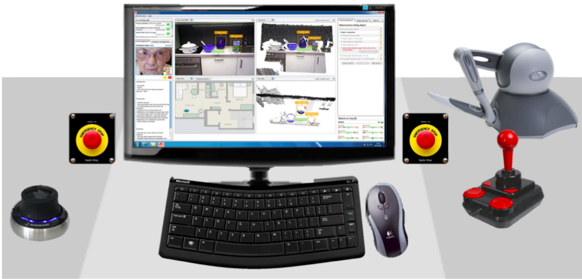
Figure 2-7: Care-O-bot 3 workstation concept for 24-hour professional teleassistant [Mast et al., 2012]. The majority of the main screen (shown in the center of the monitor) is dedicated to manipulation assistance with multi-degree of freedom devices such as the Phantom Omni (right) and SpaceNavigator (left). The prototype interface features a map of the environment overlaid with the localized robot in the bottom left of the main screen. A conventional joystick is used for controlling the robot’s navigation. The workstation includes two emergency stop buttons.
