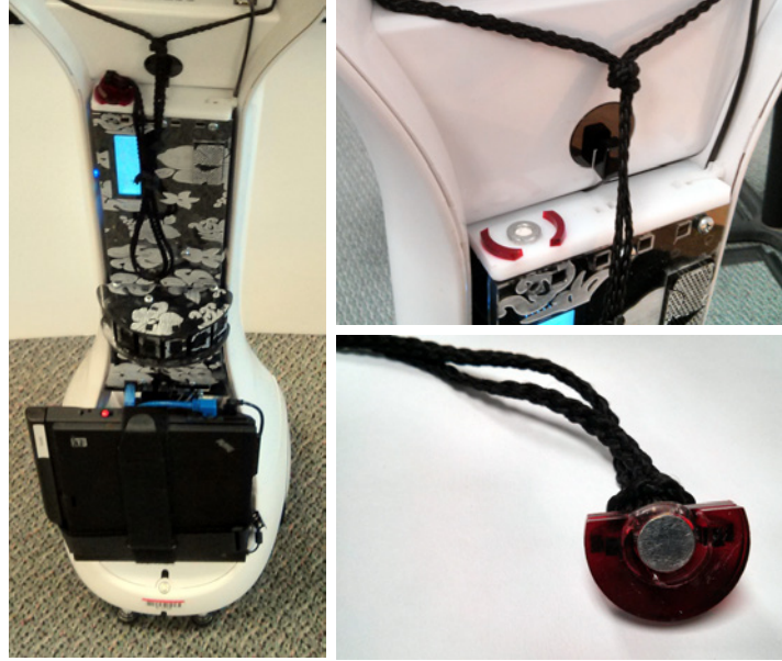
Figure 3-6: Margo emergency stop and laptop augmentations. The e-stop engages when the lanyard is pulled, similar to a snowmobile or jetski throttle kill ripcord.
