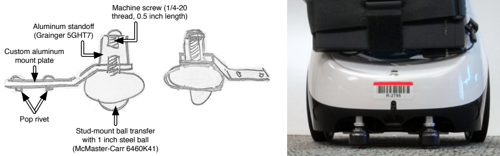
Figure 3-7: Margo rear caster replacement featuring stud-mount ball transfers.
