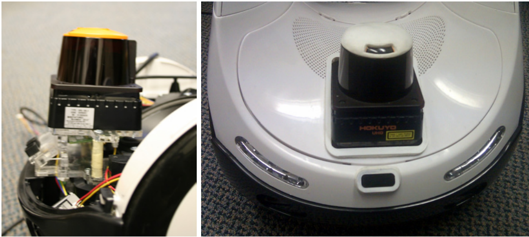
Figure 3-9: (Left) The Hokuyo UGH-08 laser is mounted in the forward center of the VGo robot's base over the base speaker. (Right) The laser's formerly orange cap has been covered with white silicon Sugru to visually minimize it.
