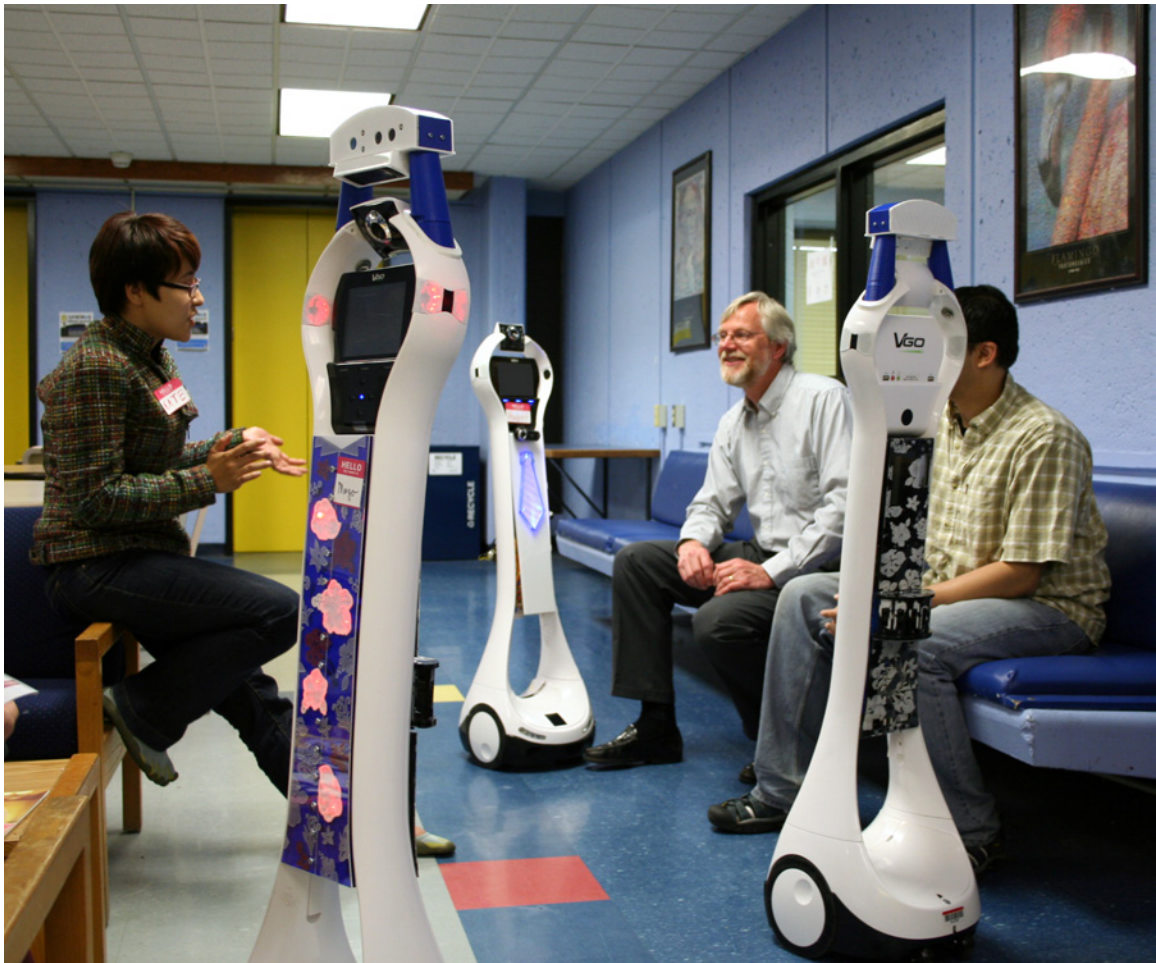
Figure 3-8: Margo (leftmost robot) exhibiting the front view of our resulting design with red LEDs lit in the shirt. View of the back panel on a sibling robot, Largo (rightmost robot).
