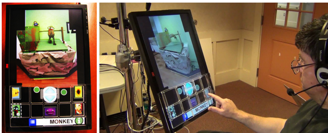
Figure 5-5: (Left) A custom clear acrylic keyguard is shown over the lower third of the interface with cutouts for the exhibit buttons, step buttons, area around the robot base icon, menu button, and iButton. (Right) The 22" monitor (shown with keyguard) was mounted on an Ergotron cart with an adjustable swing arm, which allowed it to be placed in a manner that was comfortable for the user to see and manipulate.
