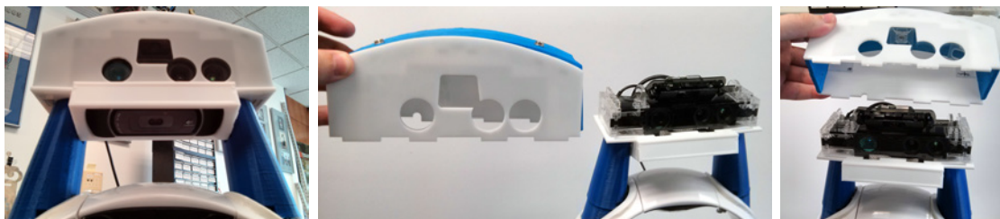
Figure 3-3: Margo's hat design features three cameras rigidly mounted together. One Logitech C910 is mounted below the Asus Xtion, and the other above.
