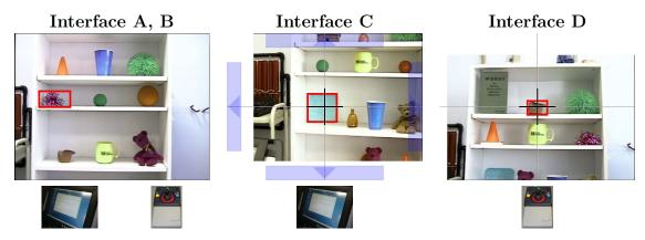
Figure 37. Object selection using our direct selection interface. The fixed camera view selection is shown on the left. The moving camera view is shown center and right, using touch screen and joystick, respectively.
