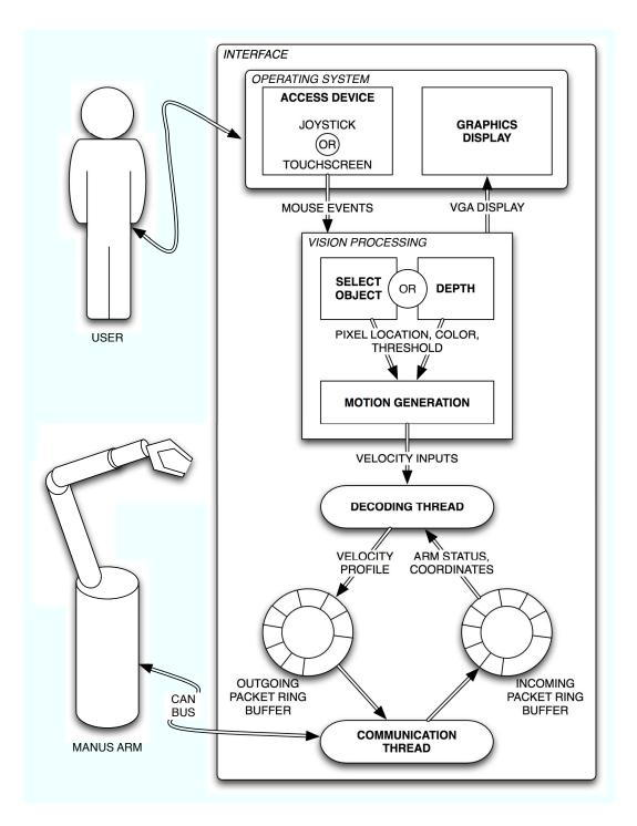
Figure 30. Data flow of our direct selection human-in-the-loop visual control system for the Manus ARM. The user provided input via touch screen or joystick mouse (top). The input was used in the vision processing (center) to position the robot arm (bottom).
