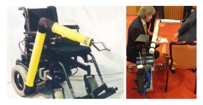
Figure 13. The Raptor Wheelchair Mounted Robotic Arm (from Phybotics 2008). The Raptor exhibited at ICORR'07 (Courtesy of Michelle Johnson).
