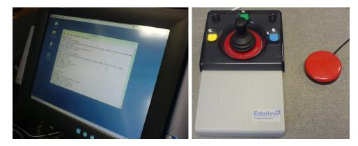
Figure 29. Our visual interface utilizes commonly used assistive technology devices such as a touch screen (left), joystick (right), and jellybean switch (far right).
