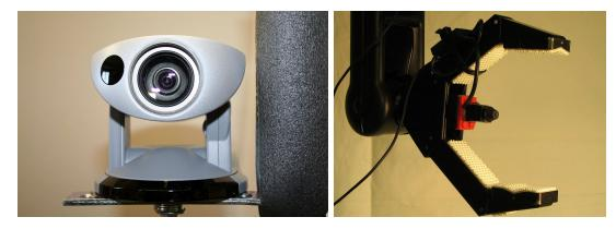
Figure 28. (Left) A Canon VC-C50i on the "shoulder" of the Manus ARM approximated the wheelchair occupant's view. (Right) A camera mounted within the gripper provided an up close view of the object to be grasped.
