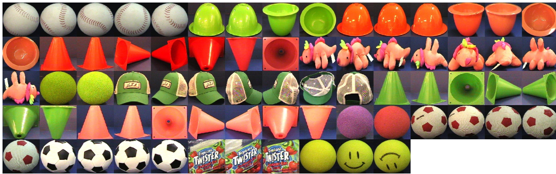
Figure 8: Input images for the neural network. These were cropped by the training program given the hand calibrated coordinates (x1,y1) and (x2,y2) that represent the top left and bottom right of a rectangle enclosing the object.
