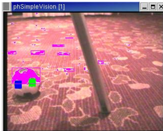
Figure 4: Soccer ball segmentation and recognition algorithm: Two black regions partially within a white region.
