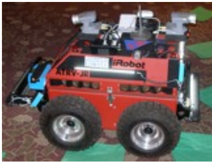
Our ARTV-JR is equipped with two pan-tilt-zoom cameras, one facing forward and one facing backward. Appropriately placed cameras can enhance an operator's awareness of the remote robot's surroundings.
