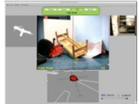
UML's USAR interface identifies a hidden victim, shown in red in the main video display. An augmented interface increases the user's situation awareness during remote operation.
