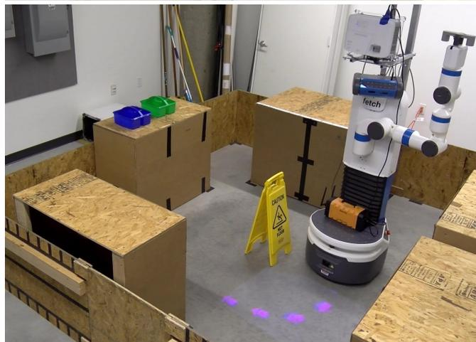
Fig. 1. A Fetch mobile manipulator navigating around a wet floor sign without (upper) and with (lower) arrow projection (purple). Despite of the effectiveness of arrow projection for revealing navigation path, no public code is readily available. Here we share such code in ROS and provide hardware support. Additional **videos** are available in [13], [14].
